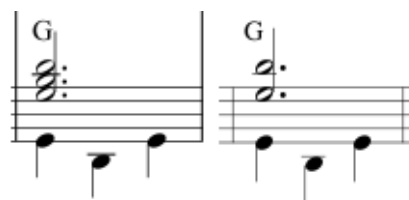
Figure 1. Example of a recognizer missing a note. Left: Bar 6 of the bass part of a piano arrangement of “God save the Queen” by T.A. Arne. Right: The output of Capella-Scan 1.6.
